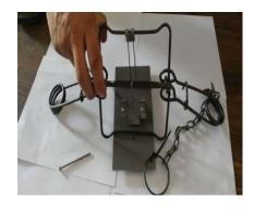
STEP 7: OPEN THE TRAP JAWS AND MOUNT THE TRAP TO THE STABILIZING PLATE AS SHOWN.
