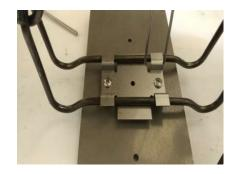
STEP 8: AT THIS POINT, YOUR TRAP SHOULD LOOK LIKE THE PICTURE. DOUBLE CHECK TO MAKE SURE SAFETY LATCHES ARE STILL IN PLACE AND THE TRAP IS IN THE BRACKET WITH THE TRIGGER LOCATED AT THE TOP.
