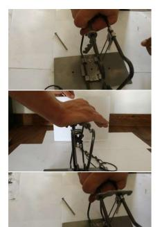
STEP 9: HOLDING THE TRAP WITH ONE HAND USE YOUR OTHER HAND TO SET THE TRIGGER. MAKE SURE YOUR TRIGGER LOCK IS IN THE MIDDLE SECTION OF THE TRIGGER SO THAT IT CAN LOCK PROPERLY.
